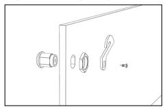
Mount the lock (4) on the front panel(1). Make sure that the hook is facing upwards in the locking position of the lock.
