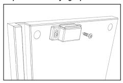
Mount the first part of the benchmagnet on the right panel (2) with existing screws.
