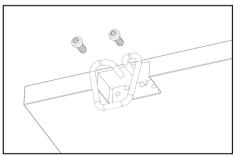
Mount the shackle (6) on the bench with the included screws. Also mount the second part of the bench magnet with the existing screws.
