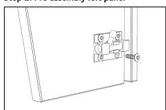
Mount the sliding lock (5) on the left panel (3) with the 4 small screws (2.5x12mm).
