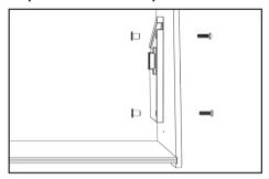
Mount the left and the right panel (2/3) in the bin with the existing screws.
