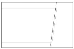
Shorten the front panel (1) by cutting the line. Tip: use a iron saw or a saw with small teeth to prevent sprintering of the wood.
